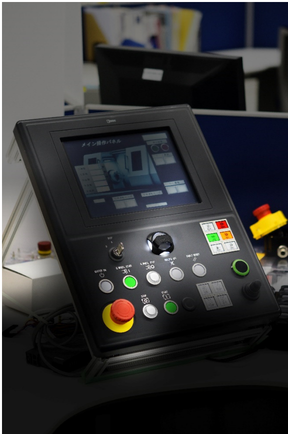
Figure 1: Unlike common commercial-grade RFID readers, industrial-rated readers are available to fit common 22mm panel-mount knockout holes while resisting harsh environments.
