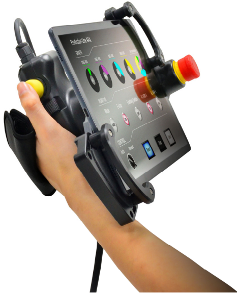
Figure 1, The IDEC HT3P Safety Commander is a unique new way to incorporate capable but relatively fragile tablets safely into an industrial automation environment.
