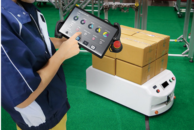
Figure 3: Robotics and AGV applications can be designed using a modern tablet-based HMI experience, yet still meet all hardwired e-stop and enable switch requirements, using the Safety Commander.
