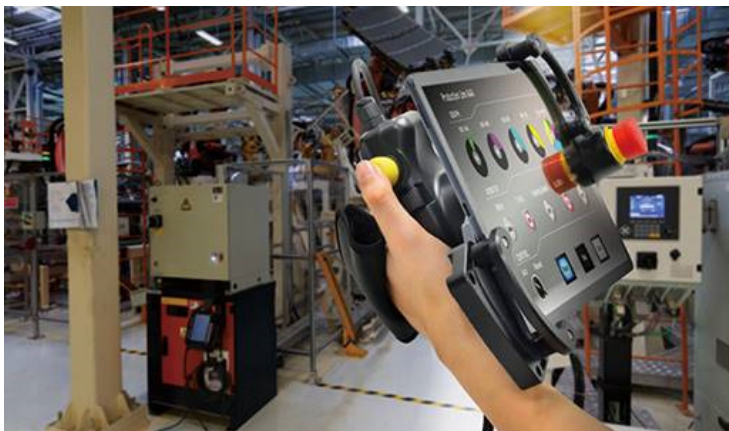
Figure 4: The ability to use tablets anywhere along a conveyance or production line gives users the best HMI options, and helps designers avoid installing excessive fixed operator interface panels.
