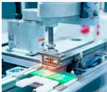
Positioning PCB conveyor lines
