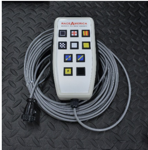
Figure 3. Handheld controllers wired to each digital safety flag allow corner operators to locally control the information displayed on the flag.
